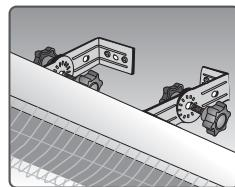
Install the two L connection parts to the back side of the heater with the screws supplied by keeping a suitable distance between them.
